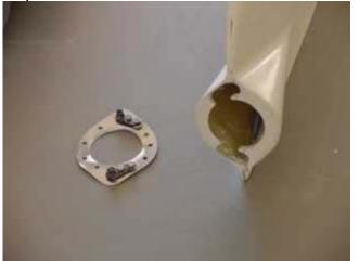
Step 6. To attach the plate to the fiberglass, use some epoxy. I drilled some extra holes in the plate to allow the epoxy to come through and create a better mechanical grip. Be sure to sand off the white gelcoat and rough up the surfaces with sandpaper. Allow to dry overnight.
