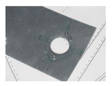
Step 3. Drill holes for the nutplates and cut the plate out of the sheet. Debur and polish it up.
