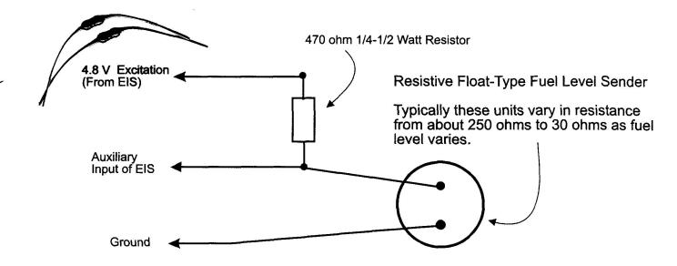
The following steps may be used to calibrate the aux display so that it displays fuel level in gallons, or any desired units.
