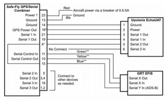
\*Rev A Safe-Fly, identified with red on label, does not support these connections. Connect EchoUAT pin 2 to aircraft power, and pin 5 directly to EFIS serial input.
