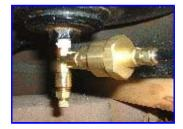
Finally, success! No leaks. The automatic drain gives a satisfying "pfft" whenever the compressor cycles on or off. The spiders can live down there in peace now...
